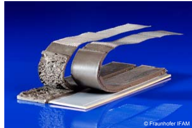
cohesive fracture / adhesive fracture
